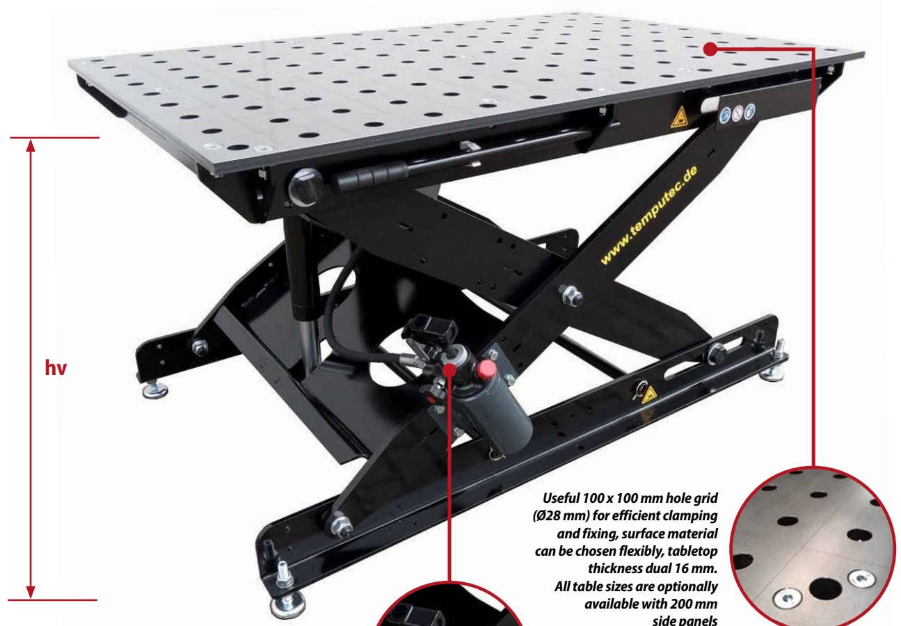
S Pic.: Temputec SST 65-105/16 S with hydraulic height adjustment from 650 to 1,050 mm, plate dimensions 1,400 x 900 mm, standard color black
